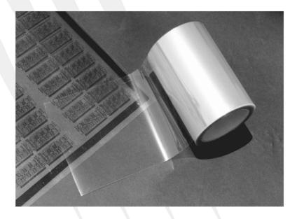
The APF-NS Protection film is a 0.5 mil. (12 microns) thick polyester film developed to protect phototools used in conjunction with liquid solder resists but is also ideal for primary image films. The smooth, non-stick coating prevents particles of photo resist from adhering to the phototool, while minimizing the need for cleaning and inspection. Ideal for track and gap widths down to 0.3 mil (8 microns). The film is completely removable without leaving any adhesive residue.
