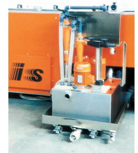
Slurry tank mounted on wheels, equipped with reclamation system, suitable for operation with different kinds of abrasive mediums such as pumice and aluminium oxide.
