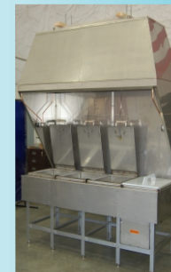
Externally Heated Tanks
