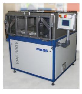
This equipment is designed for pcb via hole filling, through holes and blind vias.
